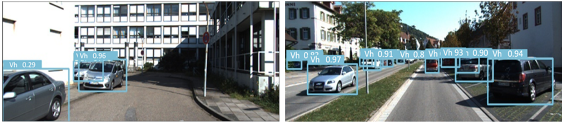
Figure 5: Vehicle detection results based on test images of KITTI dataset by using FlexiNet
