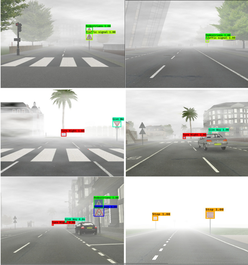
Fig. 8. The results of traffic sign recognition based on FRIDA dataset by using YOLOv5
