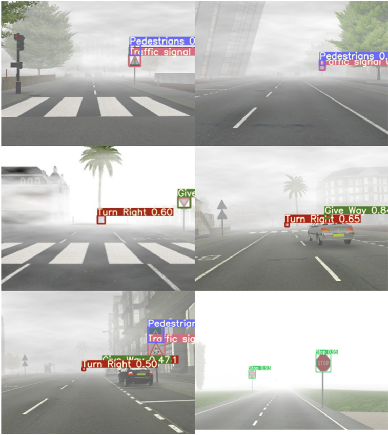
Fig. 9. The results of traffic sign recognition based on FRIDA dataset by using faster R-CNN
