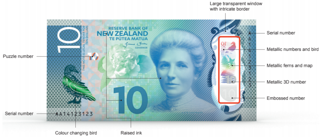
Figure 1.1 Different security features of currency. The highlighted window is our detecting target.
