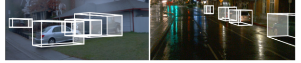
Fig. 12. The test results of 3D car detection based on the Waymo dataset by using the proposed model.
