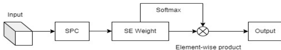
Figure 4.3 The structure of the PSA module
