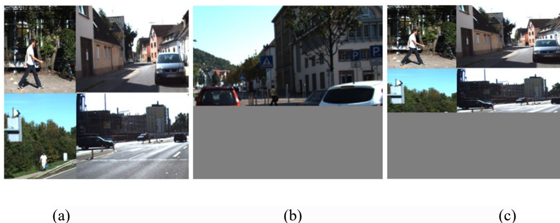
Fig. 6.4: Data augmentation in the proposed network, (a) Mosaic data augmentation where four images are merged into one frame, (b) Cutmix augmentation, where a part of the image is cut for regularization, (c) Final image produced with the combination of Mosaic and cutmix augmentation.
