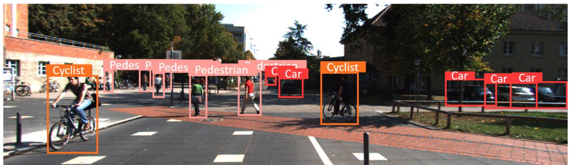
Fig. 4.7: Bounding boxes drawn around cars, pedestrians, and cyclists illustrate that every class holds a different aspect ratio, and their sizes vary w.r.t distances.
