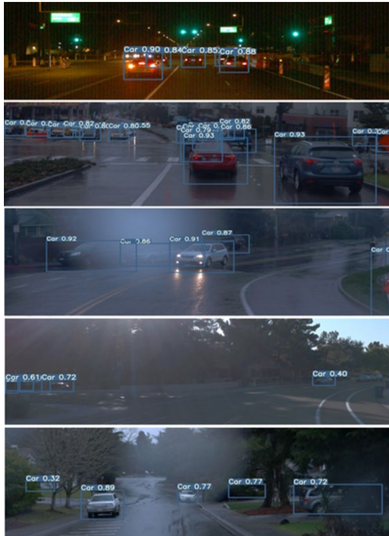
Fig. 6.20: Vehicle detection results based on test images of Waymo dataset by using FlexiNet
