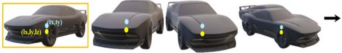
Fig. 5.7: The blue dots represent 2D centres of predicted 2D bounding boxes whilst the yellow dots refer to the 3D outermost point on the central vertical axis on the car's surface. In the right arrow shows the reference direction. Note: from (Mehtab et. al., 2021) In: ICVNZ
