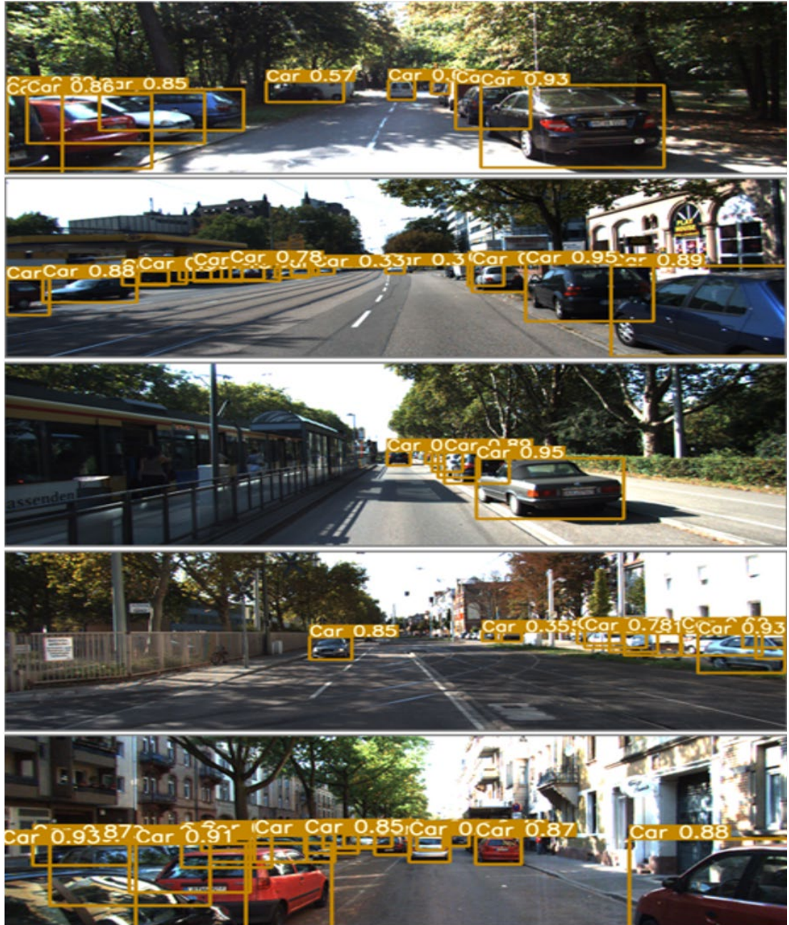
Fig. 6.18: Vehicle detection results based on test images of the KITTI dataset by using FlexiNet
