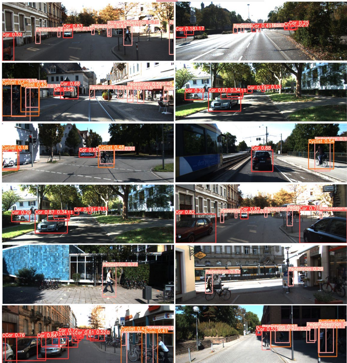
Fig. 6.13: The detection results of car, pedestrian, and cyclist instances by using the proposed FlexiNet architecture based on the KITTI dataset, from (Mehtab and Yan, 2021) In Multimedia Tools and Applications
