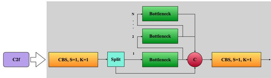
Fig 4. The structure of C2f module
