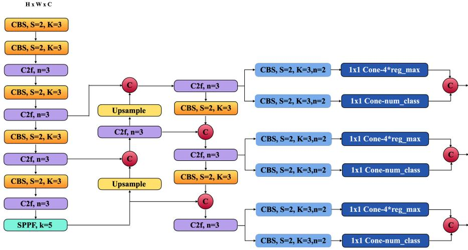
Fig 2. The structure of YOLOv8 model
