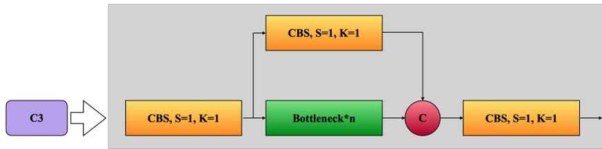
Fig 3. The structure of C3 module
