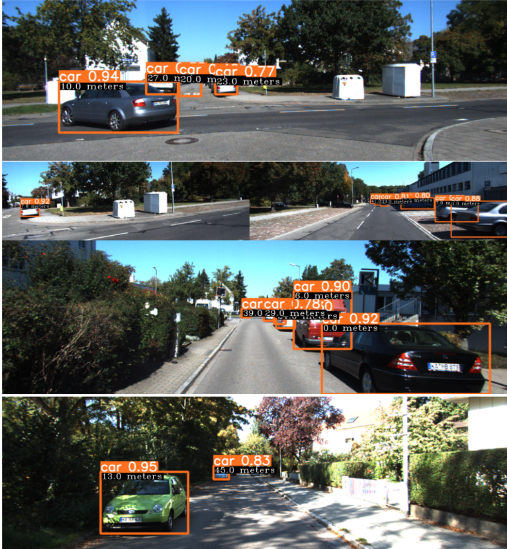
Fig. 3 The example of vehicle detection and distance estimation using YOLOv7-CBAM-Transformer
