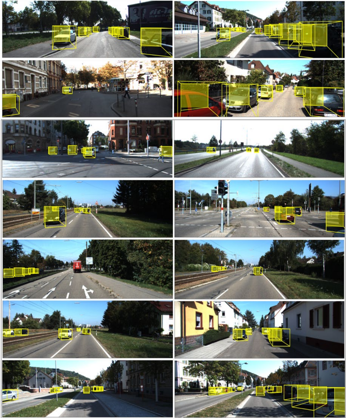
Fig. 6.26: The test results of 3D car detection based on the KITTI dataset by using the proposed model
