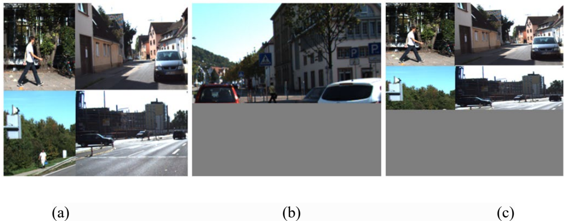
Fig. 6.4: Data augmentation in the proposed network, (a) Mosaic data augmentation where four images are merged into one frame, (b) Cutmix augmentation, where a part of the image is cut for regularization, (c) Final image produced with the combination of Mosaic and cutmix augmentation.
