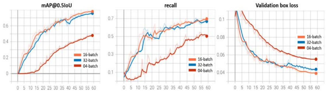
Fig. 6.6: FlexiNet performance on various batch sizes based on Adam Optimizer with finalized network size. Note: from (Mehtab and Yan, 2022) In Multimedia Tools and Applications
