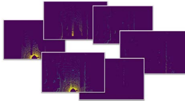
Fig. 2.2: BEV point cloud mapped in six channels based on different height levels and points' density.
