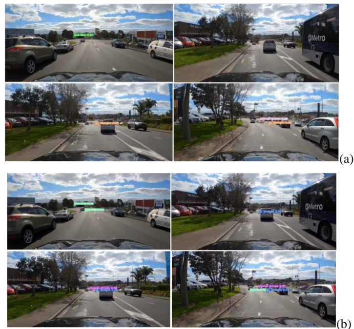
Fig.3. The TSR results on sunny days (a) Faster R-CNN (b) YOLOv5.
