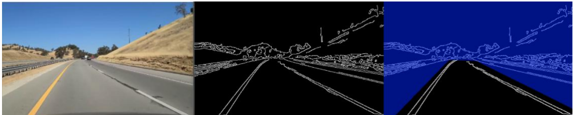
Figure 4.5 canny edge detection: original image, converted line drawing and mask
