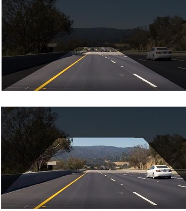
Figure 3.7 Frame mask for Hough Transform(top) and deep learning (bottom)
