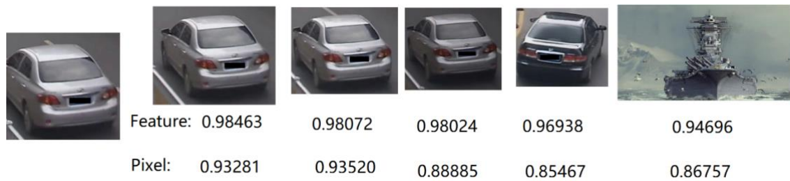
Figure 4.7 Vehicle re-id cosine distance, classification feature based and pixel based.
