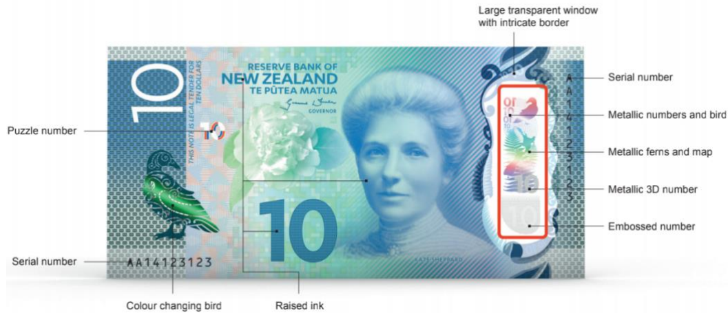
Figure 1. The security features of currency, the highlighted window is the target for object detection.
