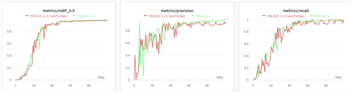
Figure 5: The comparison between YOLOv5s and YOLOv5s added Transformer
