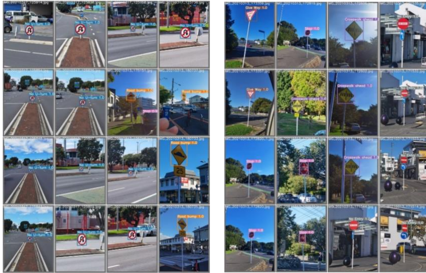
Fig.4. TSR results by using YOLOv5
