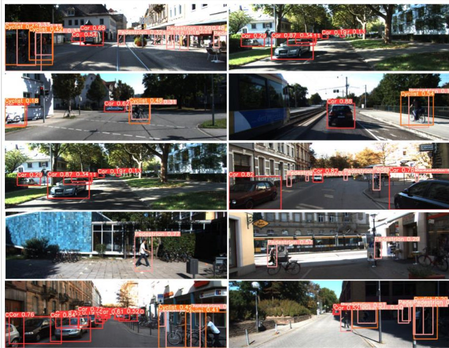
Fig. 10. The detection results of cars, pedestrians, and cyclists by using the proposed FlexiNet based on the KITTI dataset
