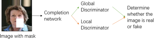
Fig. 2. Network training process. The whole network is composed of the complete network with the global discriminator and the local discriminator. These two discriminators are trained to determine the inpainted image. The completion network is trained fully for these two discriminators.
