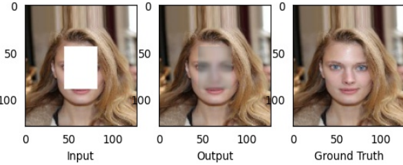
Fig. 4. Four masked positions and the corresponding results of face image inpainting. The first column is the input images with binary marks, the second column is the output result, and the third column is the ground truth.
