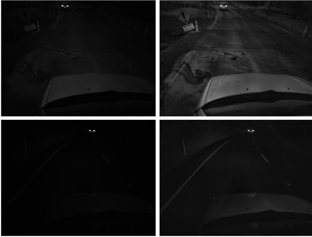
Fig. 2: *Top left*: Original image. *Top right*: Pre-processed image with sufficient quality for SGM. *Bottom left*: Very dark original image. *Bottom right*: Pre-processed image with very poor quality for subsequent processing
