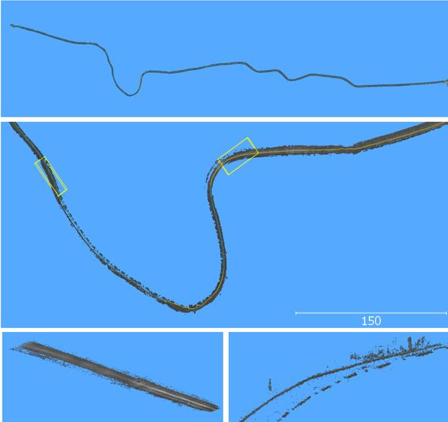
Fig. 7: *Top*: 3D point cloud for the whole road segment (one direction) generated from pre-processed night-time images. *Middle*: Curve segment. *Bottom*: Details for two sections of the shown road segment.
