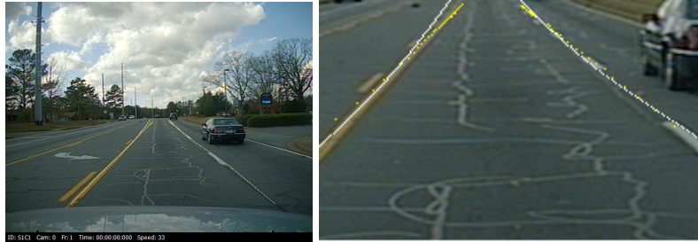
Fig. 1. Left: Ground truth and calculated lane markings. Right: Magnified window of the image shown on the left. The white lines are calculated ground truth, and the yellow dots are calculated lane-border positions. Note that algorithms for lane-border detection not necessarily provide curves; it might be just isolated dots.
