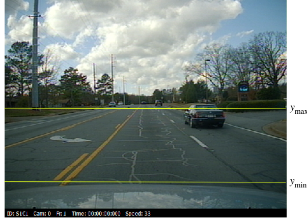
Fig. 11. Relevant rows while driving on a planar road. We are not interested in rows too close to the ego-vehicle, and not in rows too far away.
