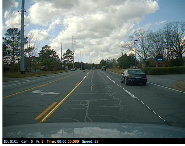
Fig. 5. Final results (white curves) after propagating points from time slices into the image sequence and interpolating those points. The image is a frame from one of the data sets provided by Borkar et al., see [2].
