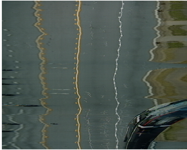
Fig. 4. Results of applying curve fitting by interpolating manually selected points to the time slice shown on the right in Figure 3. The interpolated curves are shown as thin white curves following the lane markings.
