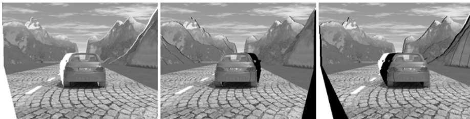
Fig. 4. Different types of occlusions for a horizontal configuration. Left: white pixels indicate occlusion between reference and match camera. Centre: black pixels indicate occlusion between third and reference camera (here: third camera is at position of match camera). Right: combined visualization where third camera is now left of the reference camera.
