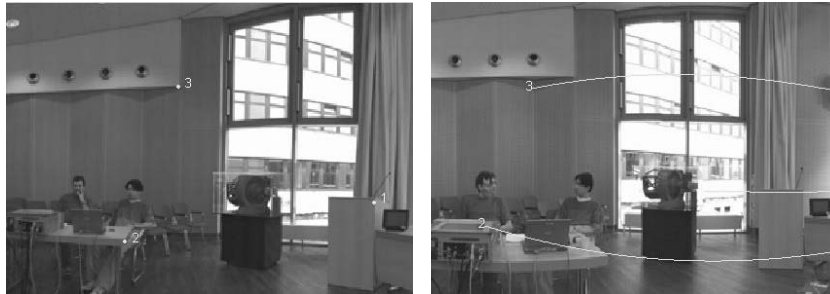
Fig. 6. Three epipolar curves calculated based on the pose estimation results.
