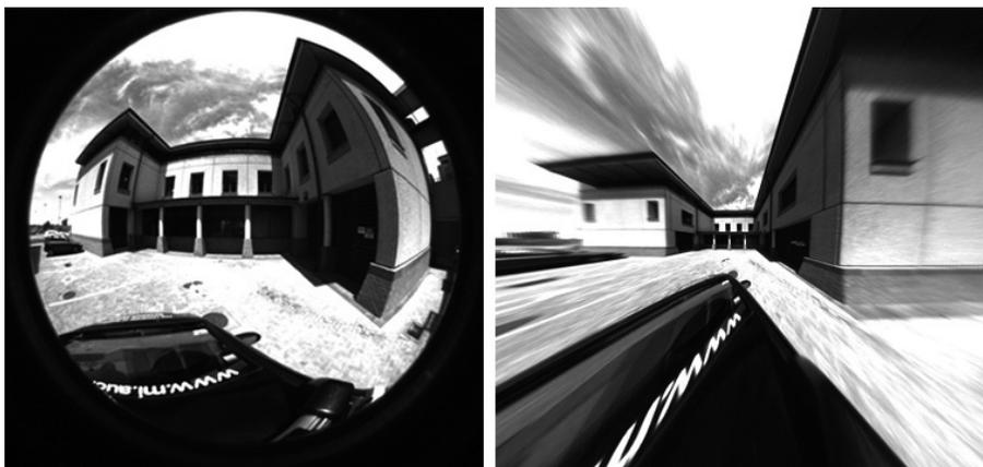
**Fig. 2.** *Left:* original fisheye image. *Right:* planar perspective undistorted image.
