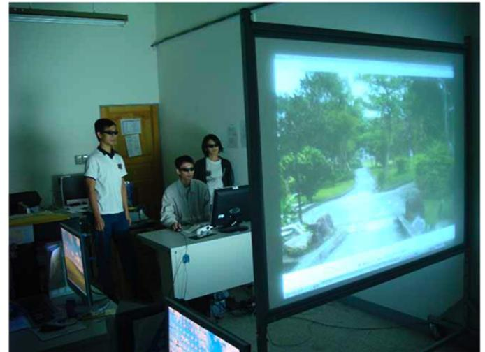
Fig. 17. The back-projection screen and polarized system for stereo panorama visualization at Ilan University, as used in the experiments reported in [27].
