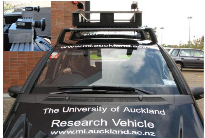
Fig. 14. Test vehicle HAKA1 of the .enpeda.. project with mounted fish-eye cameras on the roof.
