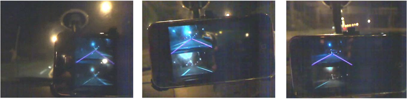
Fig. 2. Experimental results of lane detection on an iPhone at night. See [59].
