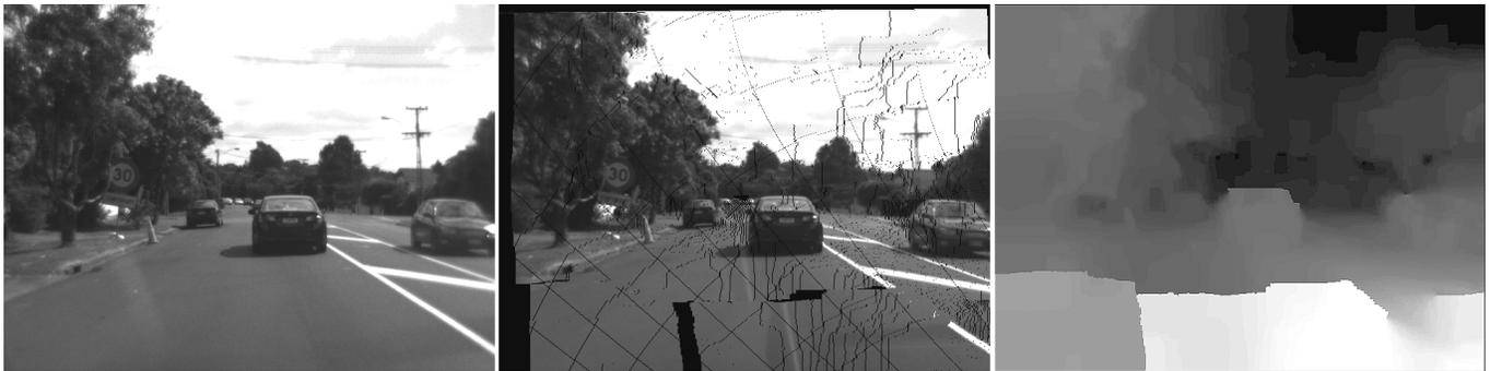
Fig. 11. An application for a trinocular sequence in Set 5 of EISATS. *Left*: third view. *Middle*: virtual view for the disparity map shown on the right. The applied matching algorithm was belief propagation stereo analysis. The specularities (see image on the left), apparent both in the recorded left and right image, causes a 'defect' in the calculated disparity data.
