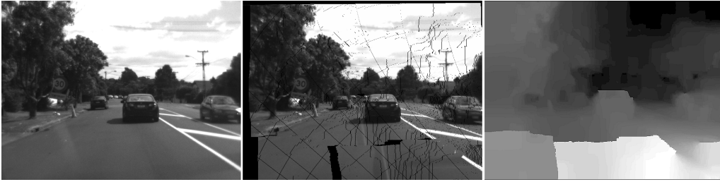
Figure 4: An application for a sequence in Set 5. Left: third view. Middle: virtual view for the disparity map shown on the right. The applied matching algorithm was belief propagation (BP) stereo analysis. The specularity (see image on the left), apparent both in the recorded left and right image, causes a ‘defect’ in the calculated disparity data.
