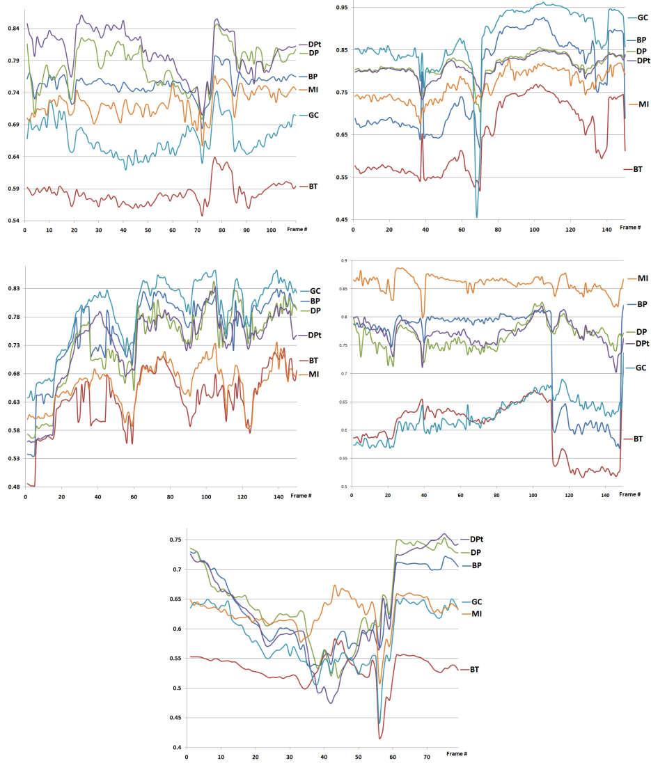
Figure 3: Performance of stereo algorithms on five different situations, using a normalized cross-correlation (NCC) measure (a larger value is ‘better’) on trinocular sequences. Top row: Left: Ordinary Conditions sequence. Right: Illumination Artifacts sequence. Middle row: Left: Inner City at Night sequence. Right: Brightness Difference sequence. Bottom: Close Objects sequence.
