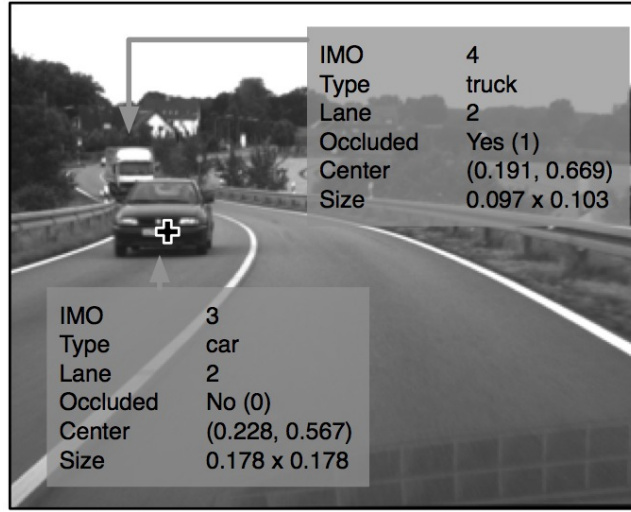
Figure 10: Frame 875 of the Suburban Bridge sequence (left camera) shows two IMOs, for which hand-labelled data are provided. Furthermore, gaze positions are available, both in coordinates and classified targets. In the ego-vehicle we observe the number plate of IMO 3 (black and white cross) and further data, also on IMO 4.
