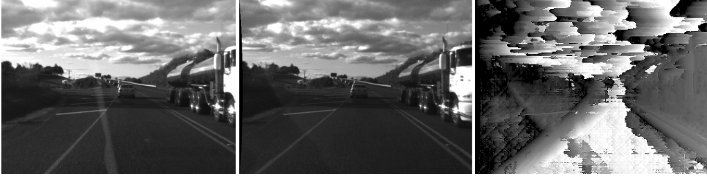
Figure 2: Example of stereo input data (left and middle) and a disparity map obtained with SGM-BT (right). This disparity map is fairly useless in this particular case; this is for illustrating a ‘bad performance’. Note that the cameras were also recording some reflections on the windscreen in this example of a situation that might be called ‘brightness differences between left and right images, and an approaching truck’; the first event (brightness differences) causes the BT cost function to fail, the second event (approaching truck) should be solvable for the SGM matching strategy in principle when using a ‘better’ cost function for matching than BT.
