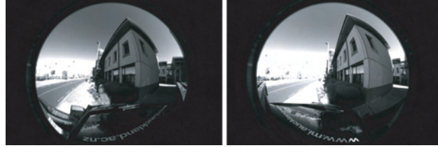
Fig. 1.7. Stereo pair of fish-eye images, for ensuring a wide field of view in vision based driver assistance.
