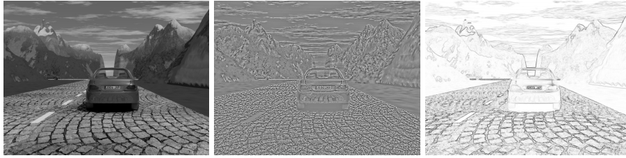
Fig. 2. Example for removing illumination artifacts due to different camera exposure in the frame 2 of EISATS set 2. Original (left) has its residual image (middle, computed using TV-L^2 ) and Sobel edge image (right) shown. Notice that the residual image retains more information than the Sobel image.
