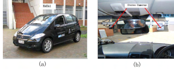
Fig. 9. (a) The test vehicle ‘High Awareness Kinematic Automobile 1’ (HAKA1). (b) A stereo camera pair on a bar behind the windscreen.
