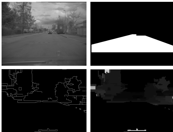
Fig. 5. The performance of the BT algorithm depends on depth discontinuities. Upper left: left image of a stereo input pair. Upper right: road mask. Lower left: depth discontinuity image. Lower right: calculated disparity map.
