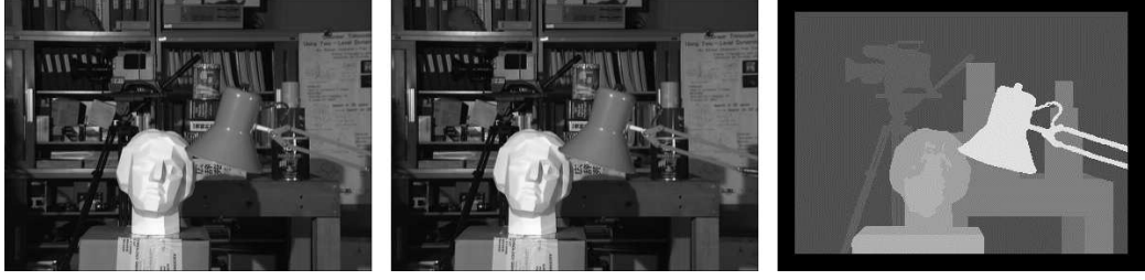
Figure 3.9: Right : An example ground truth disparity map from the Tsukuba pair. The left and right frames of the scene are pictured in the Left and Center images, respectively. Image credit : University of Tsukuba.
