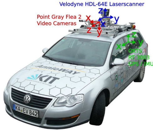
Figure 1.3: The vehicle platform used for the KITTI dataset. Image from: [41]
