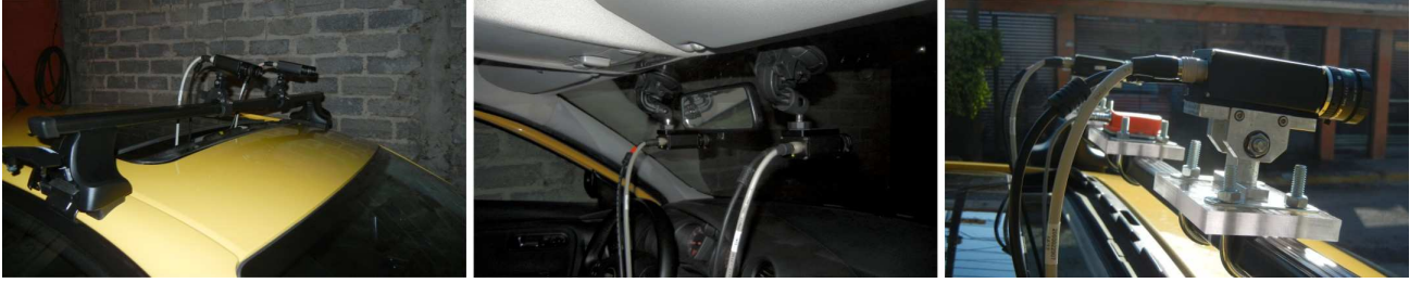
Figure 4.1: Stereo setup tests. Left : Cameras mounted using off-the-shelf camera supports. Center : Cameras mounted in the interior of the vehicle. Right : Cameras mounted using custom-made camera supports with a degree of freedom.
