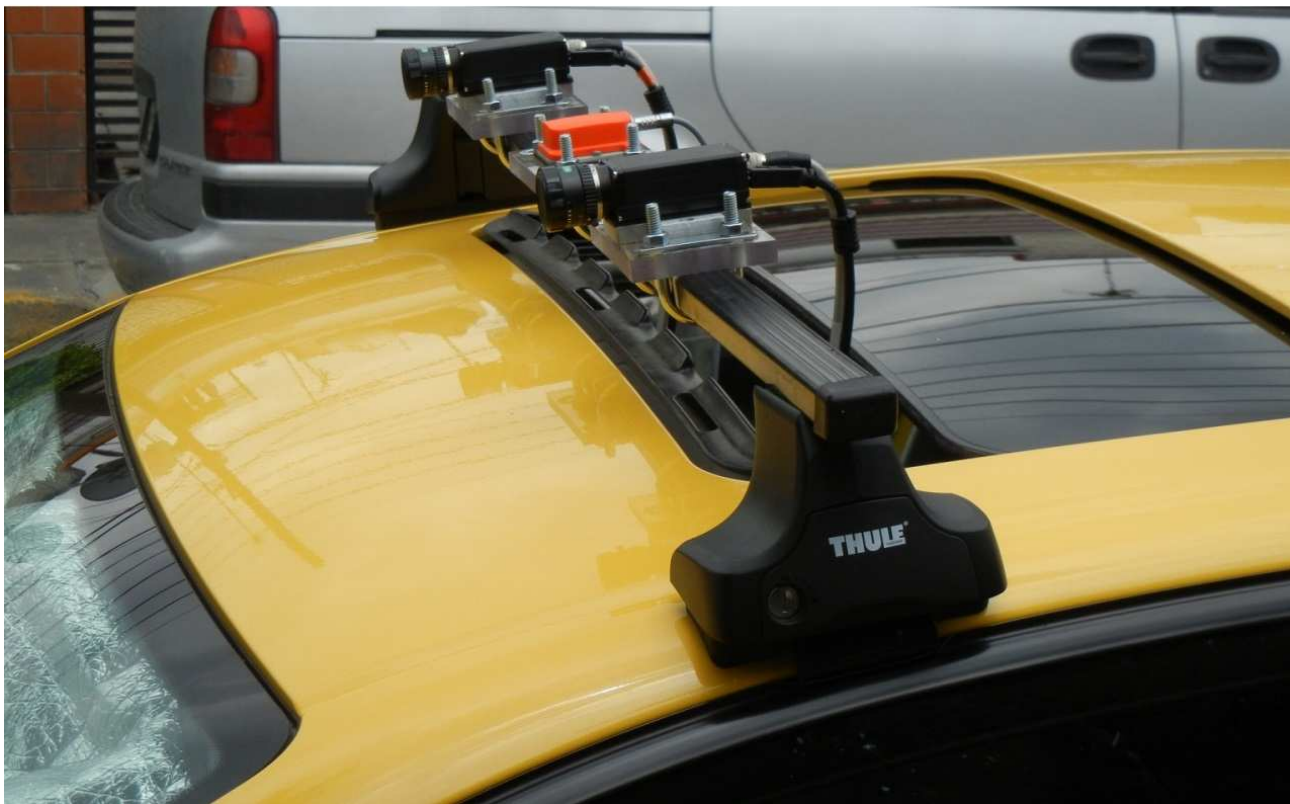
Figure 4.2: Top: A sketch of the sensor setup. Bottom: The sensor setup fixed to the vehicle. The two cameras and the Xsens MTi IMU are mounted on an bar which is then rigidly attached to the car.
