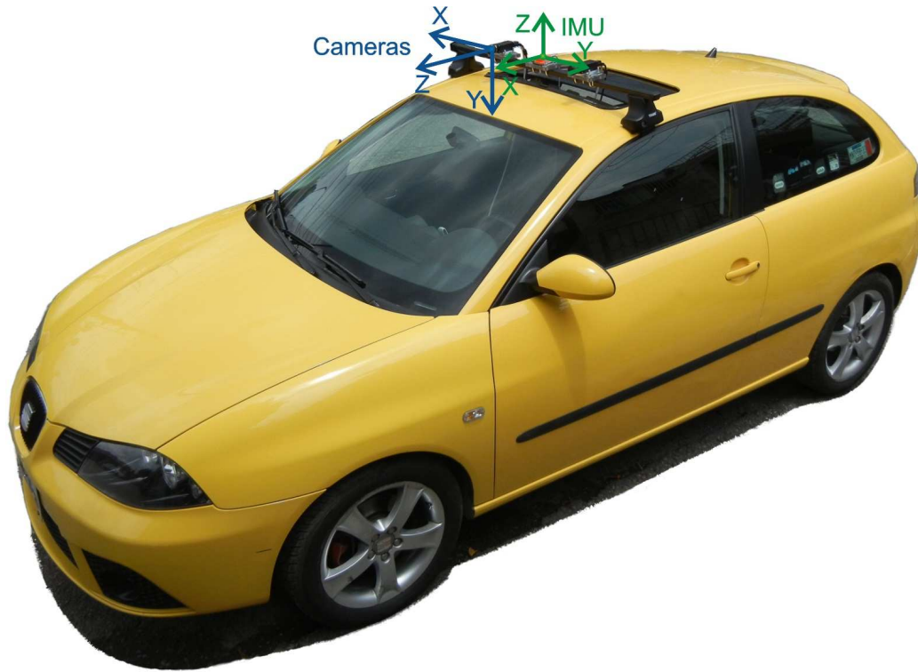
Figure 5.3: Sensor coordinate frames. The IMU coordinate frame is pictured in green, whereas the right camera coordinate frame is shown in blue.
