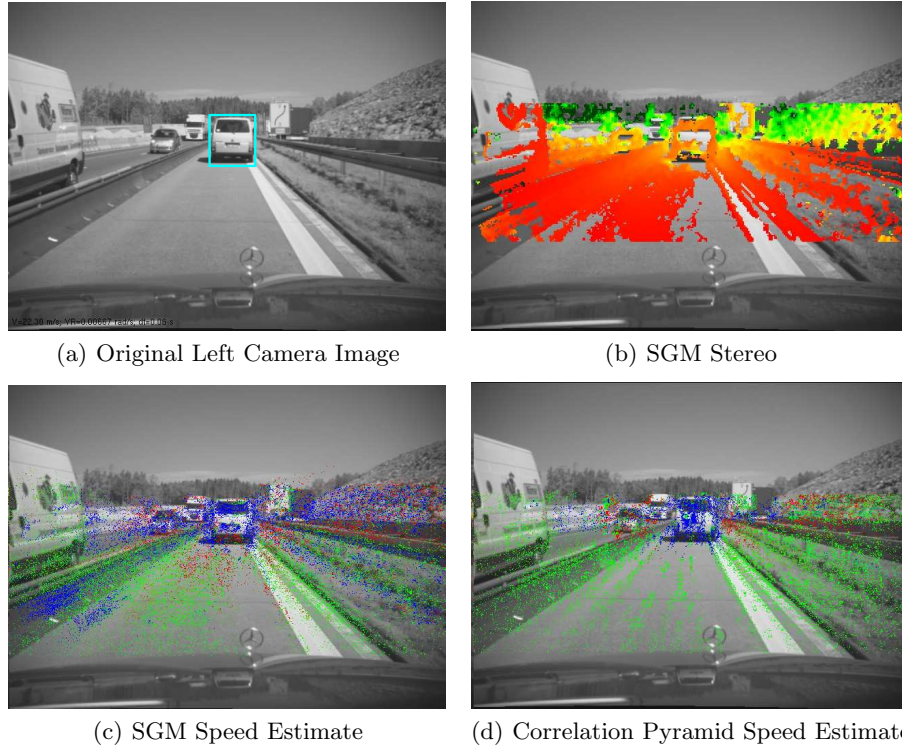
Fig. 3. Figure (b): red represents close points and green represents distant points. Figures (c) and (d): green represents static points (w.r.t. the ground), blue represents positive movement and red represents negative movement, both in the depth direction. Figure (d) shows a less noisy estimation when using Correlation Pyramid Stereo.
